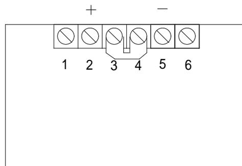
The terminals of the terminal strip are identified as the following. #1 & #6 are unused terminals. They are typically used in large arrays to feed wire through the junction box. Terminal #2 is 12 volts positive. Terminal #5 is 12 volts negative.
